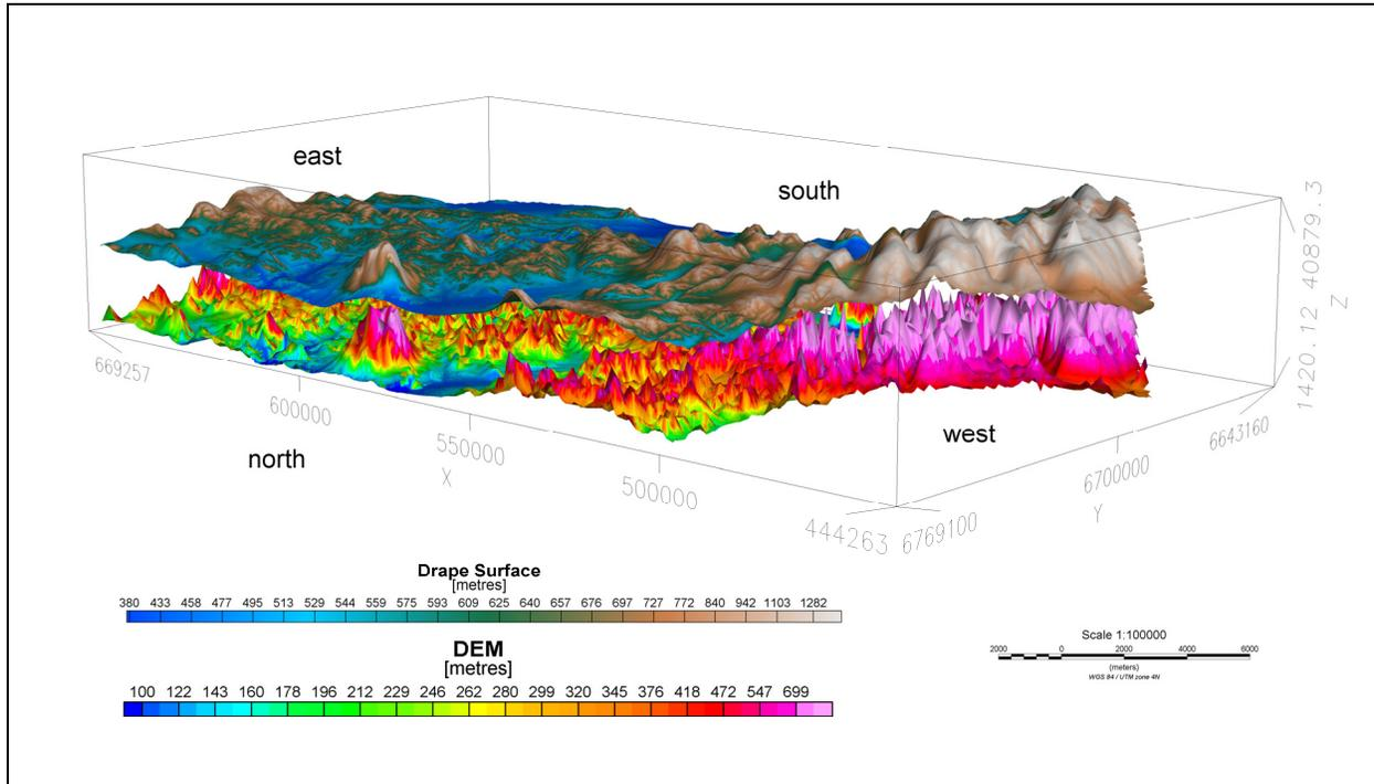
Figure 6 - view locking south-east of DEM (bottom) and Drape Surface (top)
