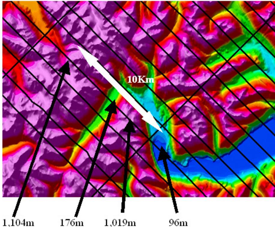
**Figure 3** - Flight path plan over DEM, showing drastic terrain variations which force to modify the survey terrain clearance
