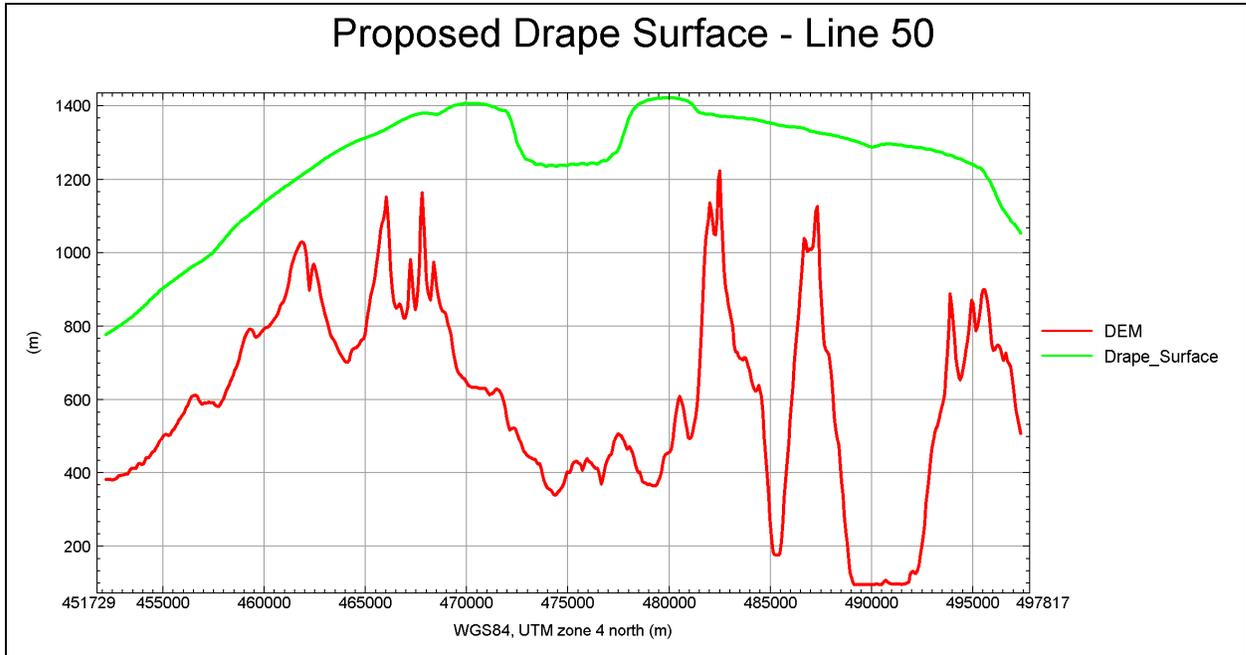
**Figure 5** - Graphical representation of DEM (red) in one of the most critical survey lines, corrected (green) to allow the aircraft to efficiently handle climb/descend angles over rugged terrain
