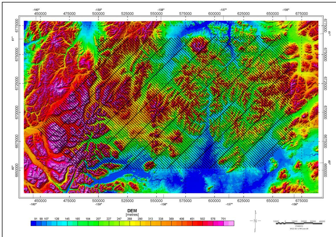
Figure 2 - Flight path plan of the survey area over Digital Elevation Model
